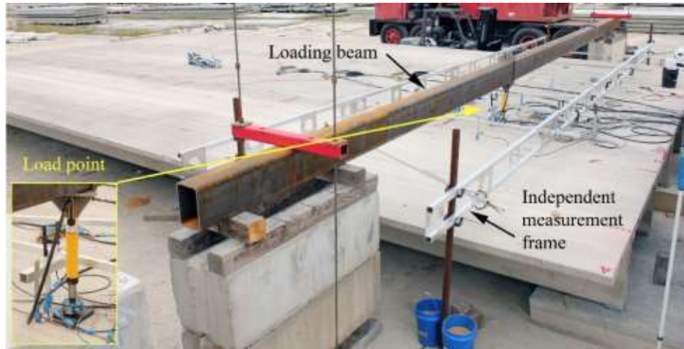
Figure 17: Testing setup on full-scale DTs for load application Bi-7.5
